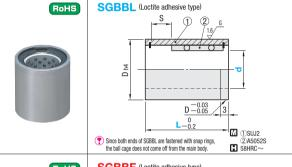
Since both ends of SGBB are fastened with snap rings, the ball cage does not come off from the main body.
