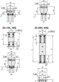
L Type Bracket Detail View The top view is Xmin and moves by slotted holes (Kx2).
