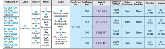
The value differs depending on the type of motor. The above values are for stages incorporating Motor F (High Torque).
