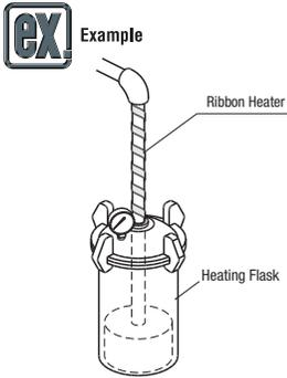
**Features:** Belt-shaped heaters easily attachable to piping and tanks.
