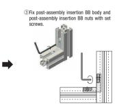
Features: Blind Brackets to connect 45 and 30 square Extrusions.
