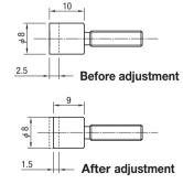
As T dimension is adjusted to be longer, it is possible to adjust it by about 1mm by cutting the bolt head as indicated above.
